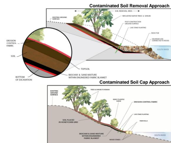
**Figure 2.** Remedial approaches for contaminated bank spoils
