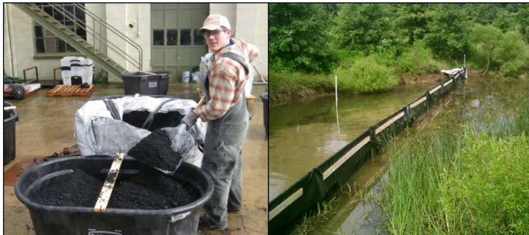
About 2,000 pounds of biochar (above left photo) were applied to one half of the pond (above right photo).
