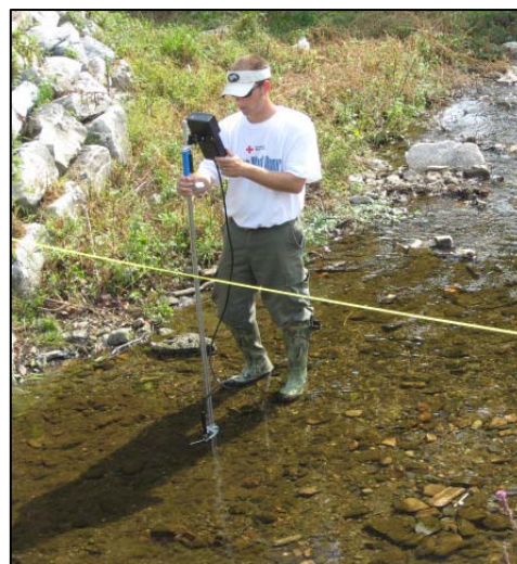
An ADV is used to measure tributary discharge.
