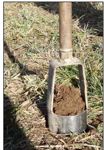
Soil samples will be collected by hand using a bucket auger.
